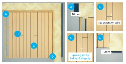
All decking materials exhibit expansion and contraction over a range of temperatures. The table below gives recommended spacing between board ends based on board length and anticipated working temperature range at time of installation.
